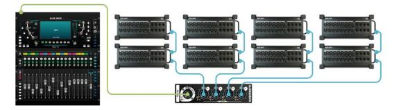
SQ + DX Hub + 8 x DX168 128 remote inputs + 64 remote outputs
