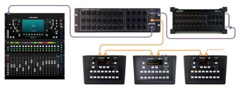
SQ + AR2412 + AB168 + ME system 40 remote inputs + 20 remote outputs + ME system
