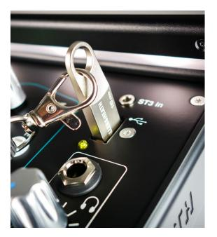
The integrated SQ-Drive makes it quick and easy to capture a 96kHz multitrack or stereo recording of the show direct to a USB key or drive.
